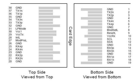
Figure 2. MSA compliant Connector
