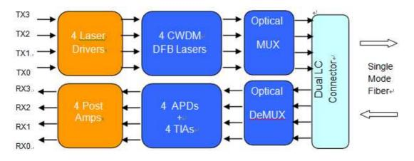
Figure 1. Transceiver Block Diagram
